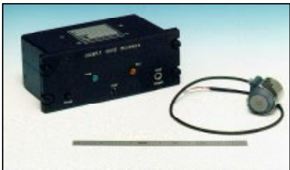
Cockpit Control Unit
