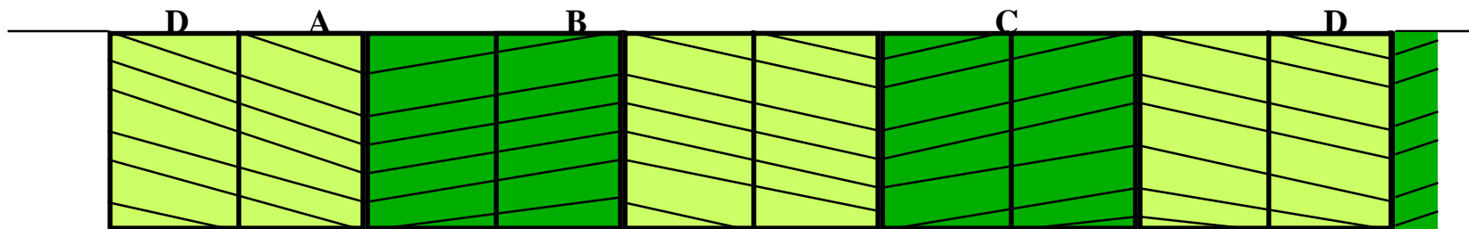
ANSI ID1 FOOTPRINT (45 \mu\text{m} pitch)
