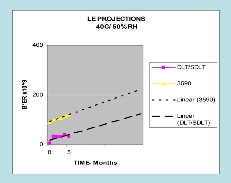
Two examples showing the LE projections using the Is projection and with ECC applied projection-note: all LE values decrease with higher temp and RH; The power of the ECC is obvious in all cases; the ECC efficiency is indicated by the difference in LE between products (best SDLT then DLT then 3590)
