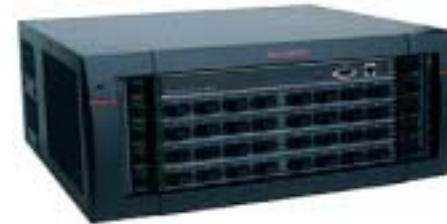
Access Hub Multi-loop hub 32 ports
