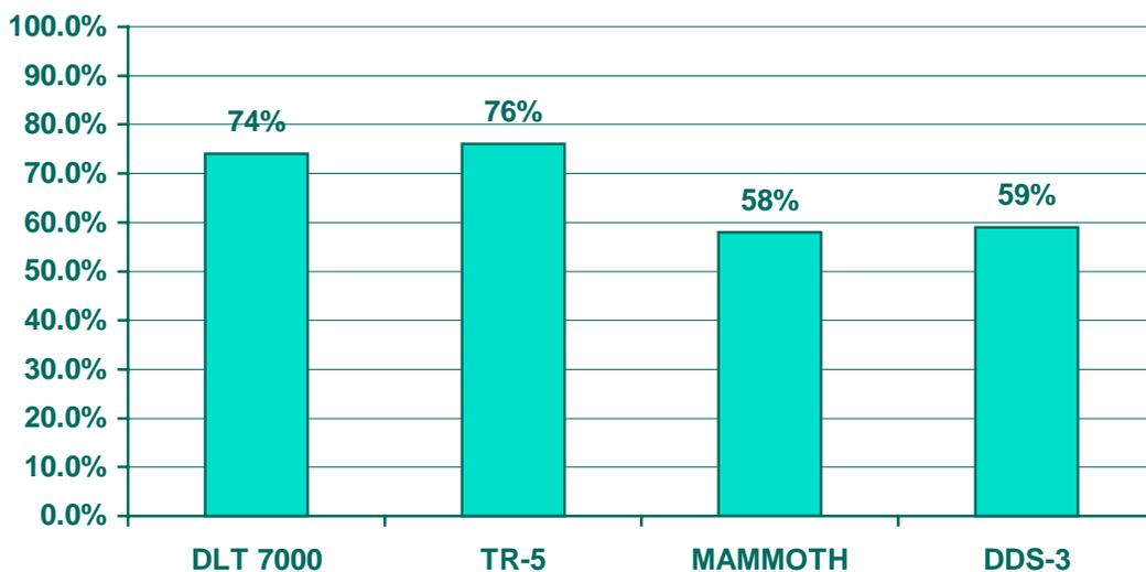
Figure 3 – Format efficiency
