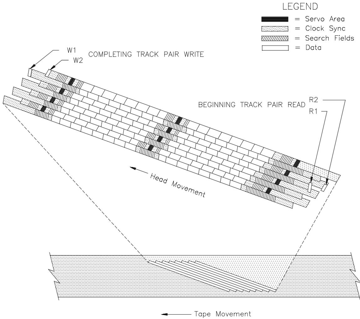
Figure 2 – Helical scan technology track format
